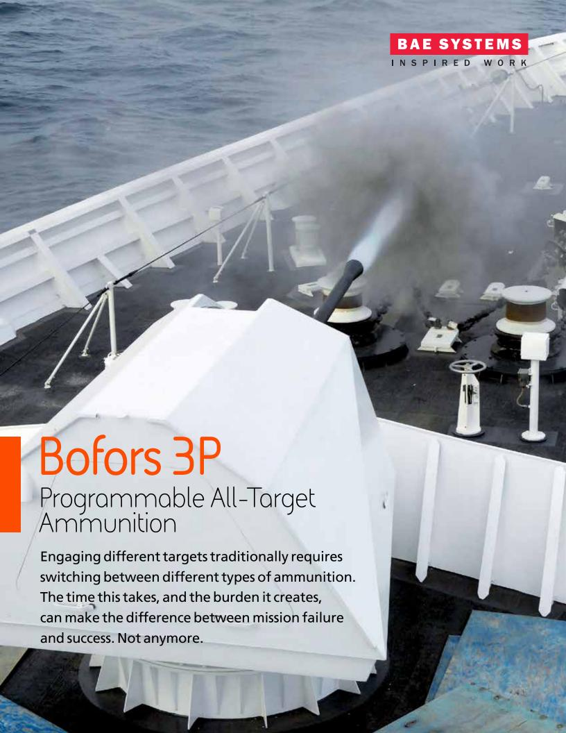
The 6-mode programmable 40 and 57 mm Bofors 3P (Pre-fragmented, Programmable, Proximity-fused) ammunition can be programmed in six different function modes to provide optimised effect against any aerial, surface or shore target. This provides weapon systems with the highest possible combat flexibility.
